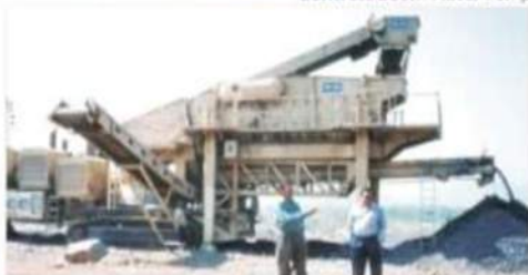
Crushing & Screening Plant
