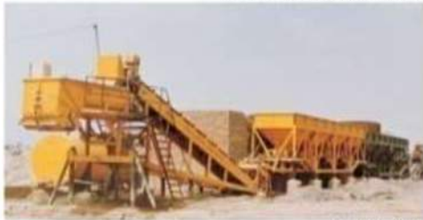
Wet Mix Plant
